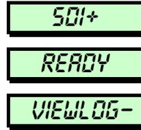
The display shows the last event recorded by the unit. In the example shown at the right, the unit sent message A to telephone number 3, which acknowledged the call.
